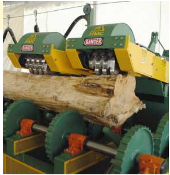
A second Debarker head is ideal for grinding knots and butt flares, while the primary head is used for routine debarking.
